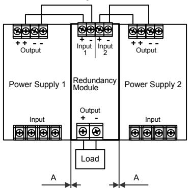
For 1+1 redundant applications, the clearance "A" can be reduced to 0mm in combination with the following power supplies:
